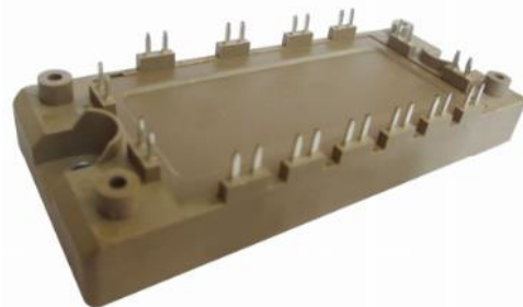
Fig. 3. GH package shape
